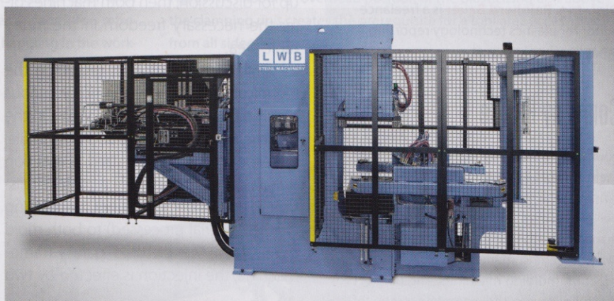
Fig. 2. Vertical, bottom-closing C-frame machine with side-extended 2500 kN clamping unit in combination with turntable unit and horizontal injection unit (© LWB Steinkl)
