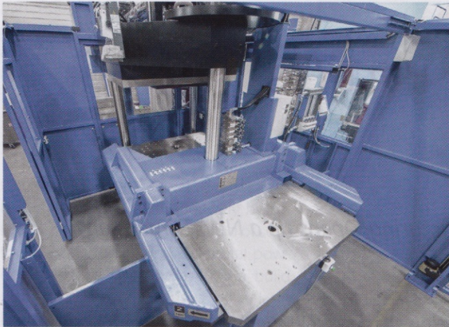
Fig. 4. Detailed view of the 3-tiebar-clamping-unit in combination with the 2-station turntable-module. The new machine concept offers maximum freedom for tool clamping and component handling in the workstation (© LWB Steinel)
